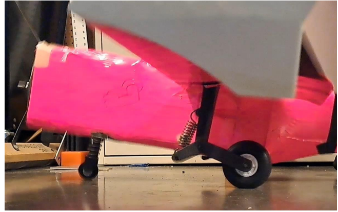
Figure 8.9.1: (left) MLG Force Vs. Stroke Plot & (right) Landing Gear Dynamic Drop Test on Prototype Aircraft
